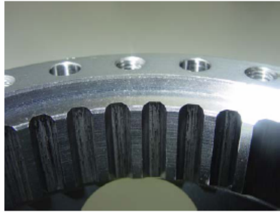
SQUARE FACE ON END OF SPLINES
